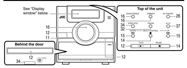
\* Connect headphones (not supplied) with a stereo mini plug. If the headphones are connected, the speakers and subwoofer will not produce any sound.
