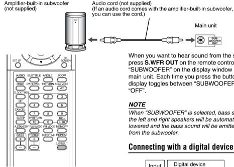
When you want to hear sound from the subwoofer, press S.WFR OUT on the remote control to display "SUBWOOFER" on the display window on the main unit. Each time you press the button, the display toggles between "SUBWOOFER" and "OFF".
