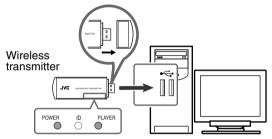
If your PC does not detect the transmitter, disconnect the transmitter and connect it again. If it does not work yet, restart Windows.
