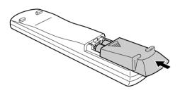
If the range or effectiveness of the remote control decreases, replace the batteries. Use two R6 (SUM-3)/AA(15F) type dry-cell batteries.
